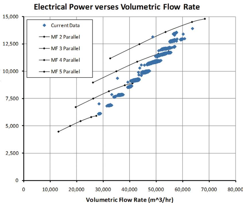
Figure 2 | Variations in Electrical Power due to Dynamic System Characteristics
