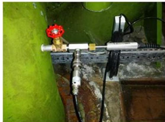
Figure 5 Hydraulic efficiency pressure and temperature transducers (104 installed)
